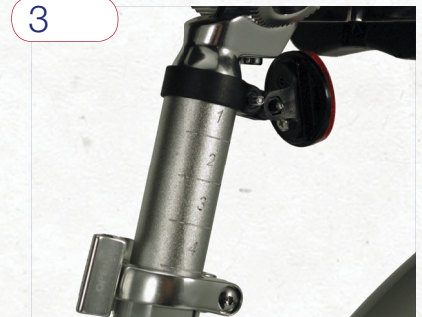
The seat post has graduated marks indicating its height. After adjustment, note your setting for future use.
